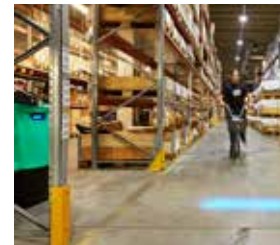
Blue point safety light towards driving direction (forks trailing).
