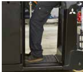
Suspended operator's platform.
